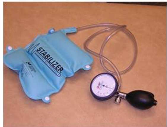
Figure 14.2 A pressure bio-feedback unit. The unit is inflated to 70 mmHg pressure and placed under the lower abdomen while the subject is lying in prone position. When the correct contraction is performed, pressure decreases by approximately 6–8 mmHg.
